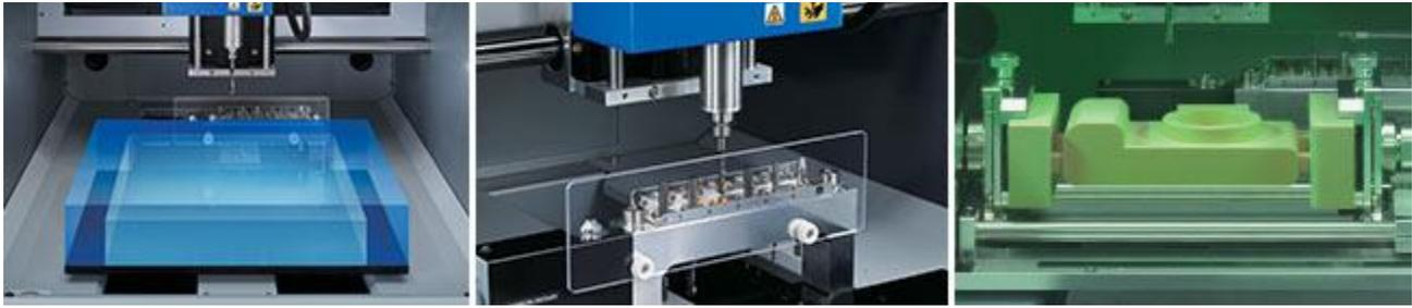
*Operating range X: 15.75in (400mm) Y: 12.00in (305mm) Z: 5.315in (135mm)*
